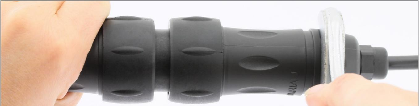
4. Control: Pull on the cable to ensure that the retention system bottoms in the backshell.
