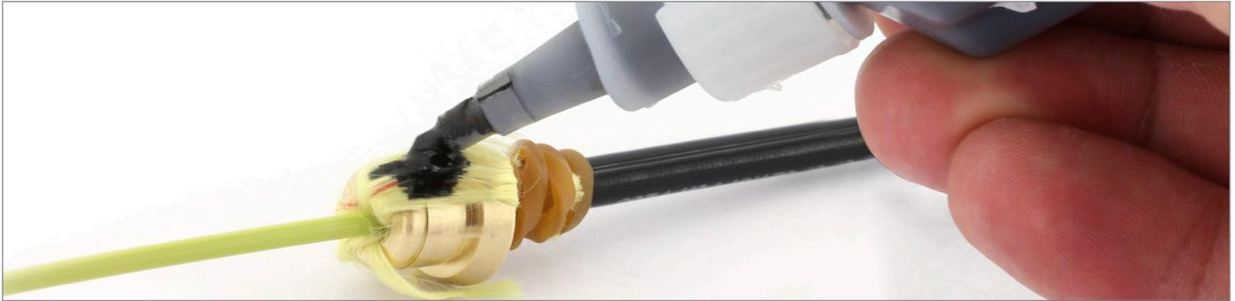
8. Before the instant adhesive begins to harden, quickly slide the ear clamp over the fiber, orient the Clamp according the picture. Push the strength members back over the clamp until it bottoms on the rear flange of the support.
