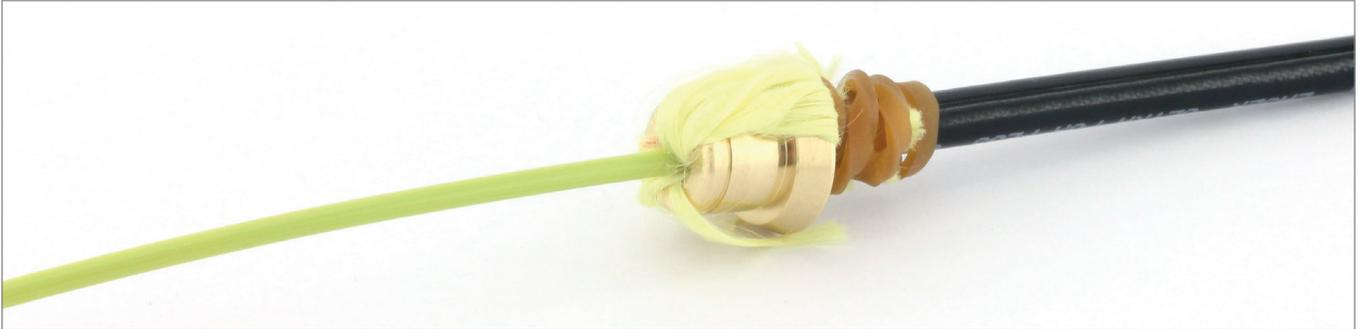
7. Apply the instant adhesive on the fiber and cover the crimp support. (e.g. Loctite 480 PRISM).
