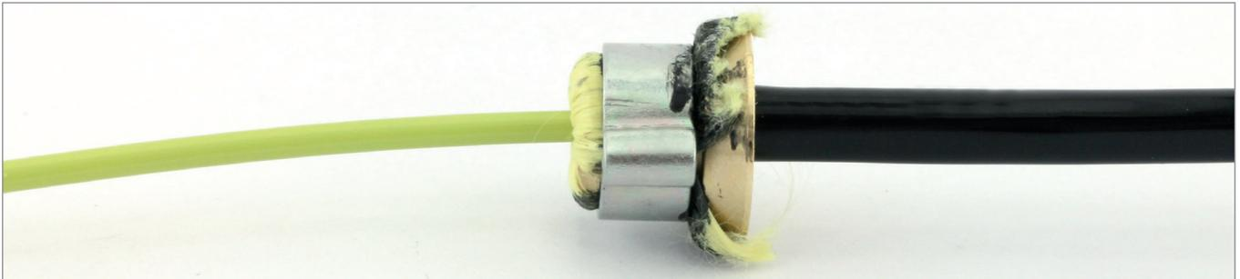
9. Crimp the both ear of the Clamp using the Nipper. Remove the kevlar strength members using using the shears.
