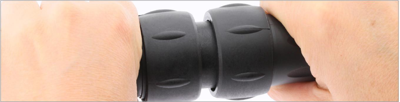
3. Slide the backshell and screw it using a 28 mm U-wrench. Tightened the backshell with a 4 Nm torque.
